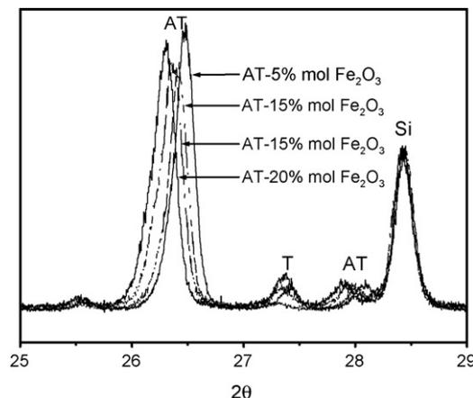
Fig. 3. XRD patterns for iron stabilized tialite (AT: aluminium titanate; T: titanium oxide; Si: silicon).
