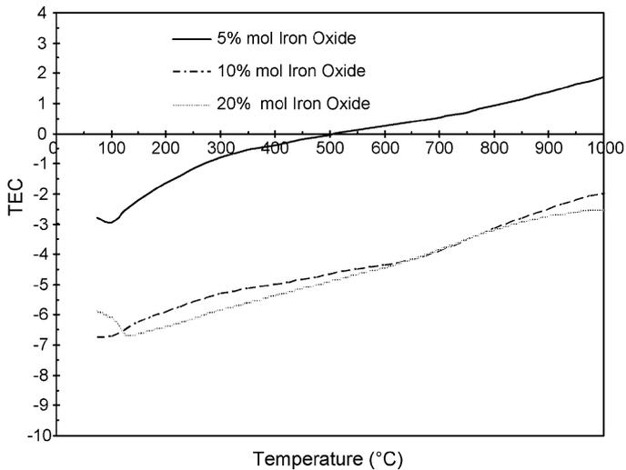
Fig. 5. Thermal expansion coefficient ( $\times 10^{-6} \text{ }^\circ\text{C}^{-1}$ ) of  $\text{Al}_2\text{TiO}_5$  stabilized with iron oxide.
