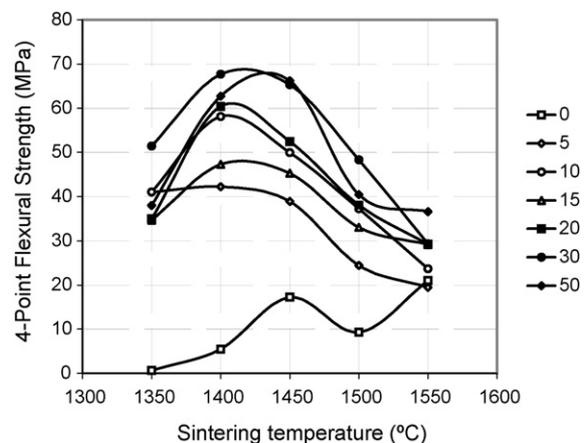
Fig. 7. Flexural strength vs. temperature for tialite (20 mol% iron oxide stabilized)–mullite composites.
