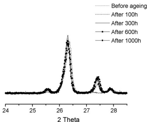
Fig. 2. XRDs of AT-20 mol%  $\text{Fe}_2\text{O}_3$  after 100, 300, 600 and 1000 h at  $1100^\circ\text{C}$ .
