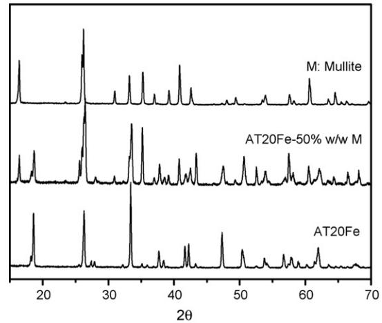
Fig. 6. XRD patterns for AT20Fe, mullite (M) and AT20Fe–50% M.
