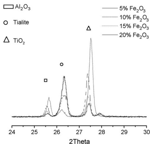
Fig. 1. XRD patterns of AT- $x$  mol%  $\text{Fe}_2\text{O}_3$  ( $x=5, 10, 15, 20\%$ ) after 1000 h at  $1100^\circ\text{C}$ .
