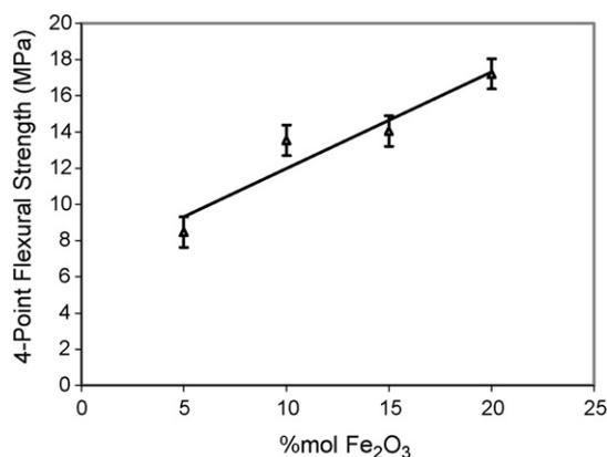
Fig. 4. Flexural strength of AT vs. mol  $\text{Fe}_2\text{O}_3$  and sintered at  $1450^\circ\text{C}$ .
