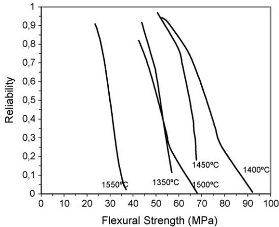
Fig. 9. Flexural strength reliability for tialite (20 mol% iron oxide stabilized)–30% (w/w) mullite composite.
