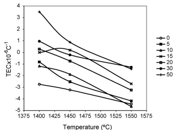
Fig. 11. Thermal expansion coefficient values for AT20Fe–mullite composites vs. sintering temperature.
