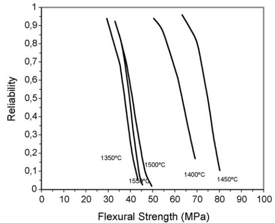
Fig. 10. Flexural strength reliability for tialite (20 mol% iron oxide stabilized)–50% (w/w) mullite composite.
