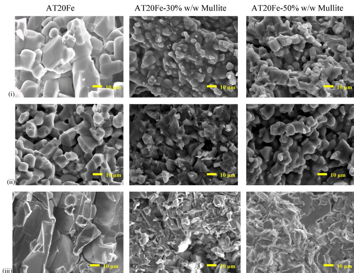
Fig. 8. SEM images ( $\times 2500$ ) for AT20Fe–mullite composites sintered at: (i) 1400 °C, (ii) 1450 °C and (iii) 1550 °C.
